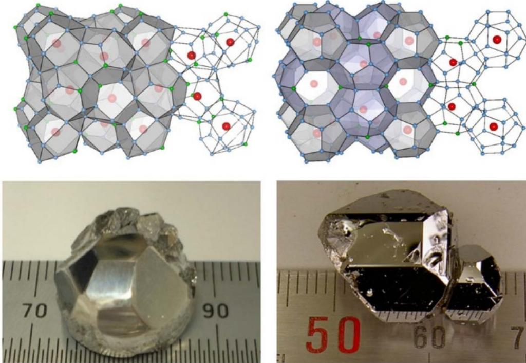
FIG. 1. (Color online) Crystal structures and corresponding as-grown single crystals of (a)  $\alpha$ - $\text{Ba}_8\text{Ge}_{16}\text{Sn}_{30}$  and (b)  $\beta$ - $\text{Ba}_8\text{Ge}_{16}\text{Sn}_{30}$ .
