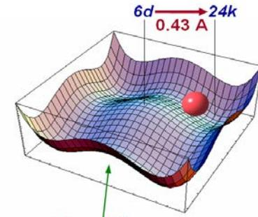
Purely theoretical approach is possible for  $T > 100\text{K}$  by taking into account the situation: Heat is carried via the cascade transfer of cage vibrations created by true rattling motion of guest atoms.
