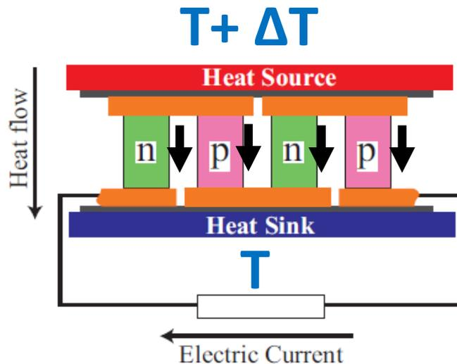
FIG. 1 (Color online) Thermoelectric devices contain many thermoelectric couples consisting of *n*-type and *p*-type thermoelectric elements wired electrically in series and thermally in parallel.
