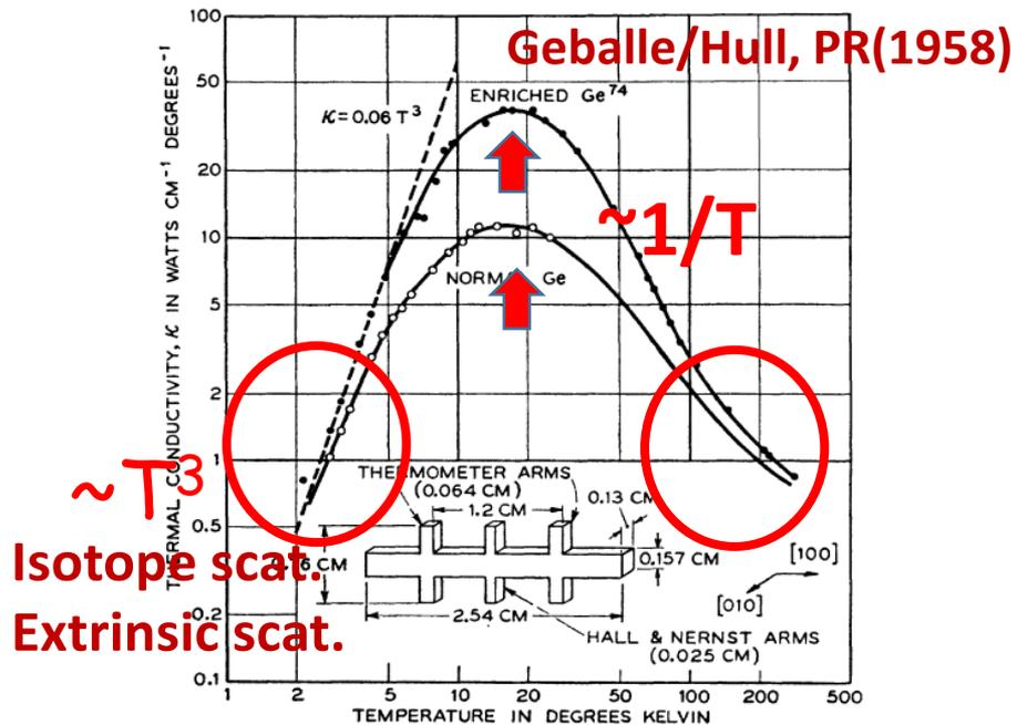
FIG. 2. Isotope effect on thermal conduction in germanium. The peak conductivity of the enriched (96%  $Ge^{74}$ ) sample is how much higher than that of the normal (96%  $Ge^{73}$ ) sample. The boundary between the two regions is in good agreement with the Casimir theory (Sec. V11) for the pure sample, but does not approach  $T^3$  variation in the normal sample even at the lowest temperatures attained.
