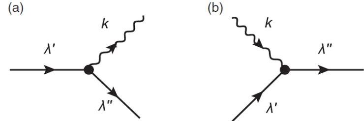
FIG. 5. The diagrams showing the hopping process for SL modes arising from anharmonic interaction between SL modes and extended modes: (a) SL  $\rightarrow$  extended + SL and (b) extended + SL  $\rightarrow$  SL. The solid lines denote the SL mode and the wavy lines the extended mode.
