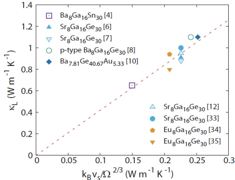
FIG. 2. (Color online) Observed  $\kappa_L$  for various off-center type-I clathrates as a function of  $k_B v_s / \Omega^{2/3}$  4,6–8,10,12,33–35. Solid inverted-triangle on off-center Eu<sub>8</sub>Ge<sub>16</sub>Sn<sub>30</sub> de-
