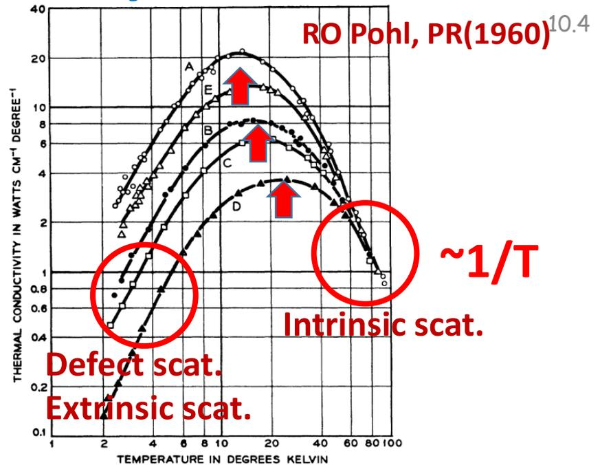
FIG. 4. Thermal conductivity of LiF as a function of temperature for various levels of irradiation. The curves are for different levels of irradiation: A,  $6.7 \times 10^{19}$  cm $^{-2}$ ; B,  $1.34 \times 10^{20}$  cm $^{-2}$ ; C,  $2.68 \times 10^{20}$  cm $^{-2}$ ; D,  $5.36 \times 10^{20}$  cm $^{-2}$ ; E,  $1.07 \times 10^{21}$  cm $^{-2}$ .
